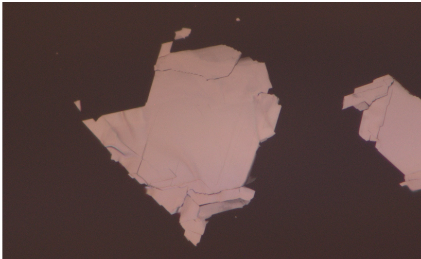
Figure 9: Example of one of the PtSe 2 flakes used to calculate contrast.
