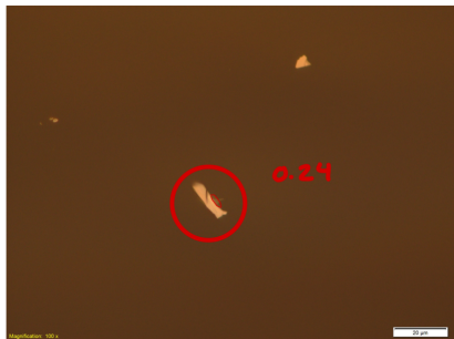
Figure 11: Monolayer found after calculating the chi-square predicted value, falls within reasonable contrast uncertainty from prediction.
